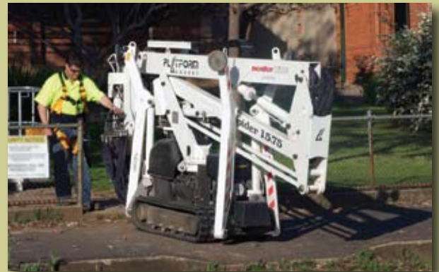
Reduces to only 780mm wide and lowers to 1909mm height for narrow access.
