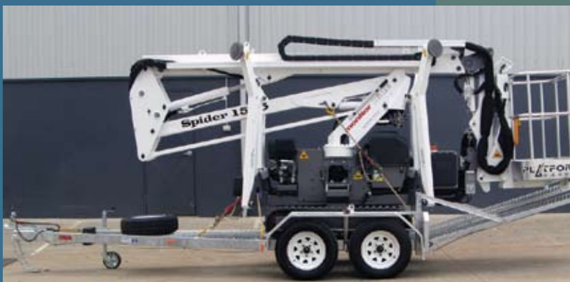
Total package weight with heavy duty gal. steel trailer: 2590kg
