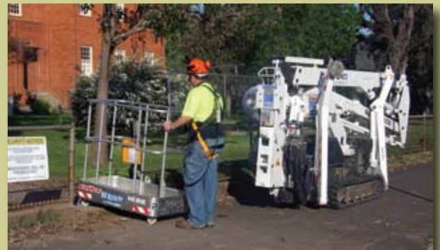
Platform quickly and simply detaches with only one pin for accessing very tight locations.
