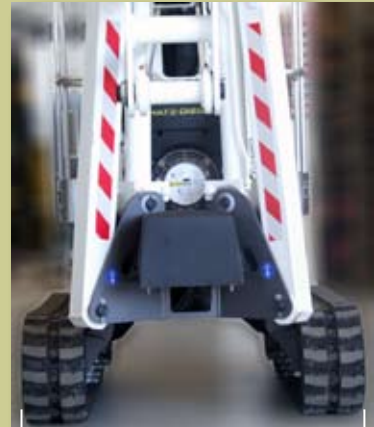
Expands to 1060mm for extra stability and stands taller for extra off-road clearance.
